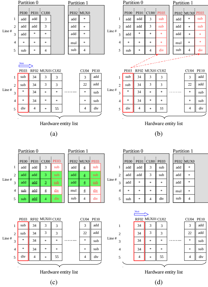
Fig. 2. Packing Process of compression technique
